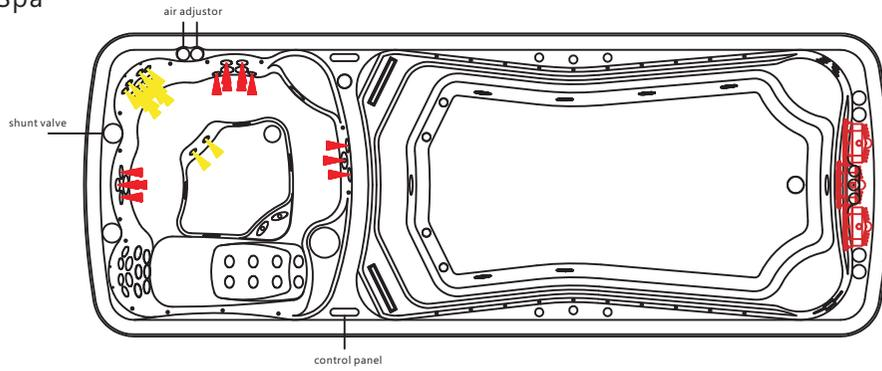
1. Turn on the Surfing pump1. Mainfold contrarotate ■ spray water, Clockwise Rotation ■ spray water Mainfold pointer in the middle ■ & ■ spray water together
