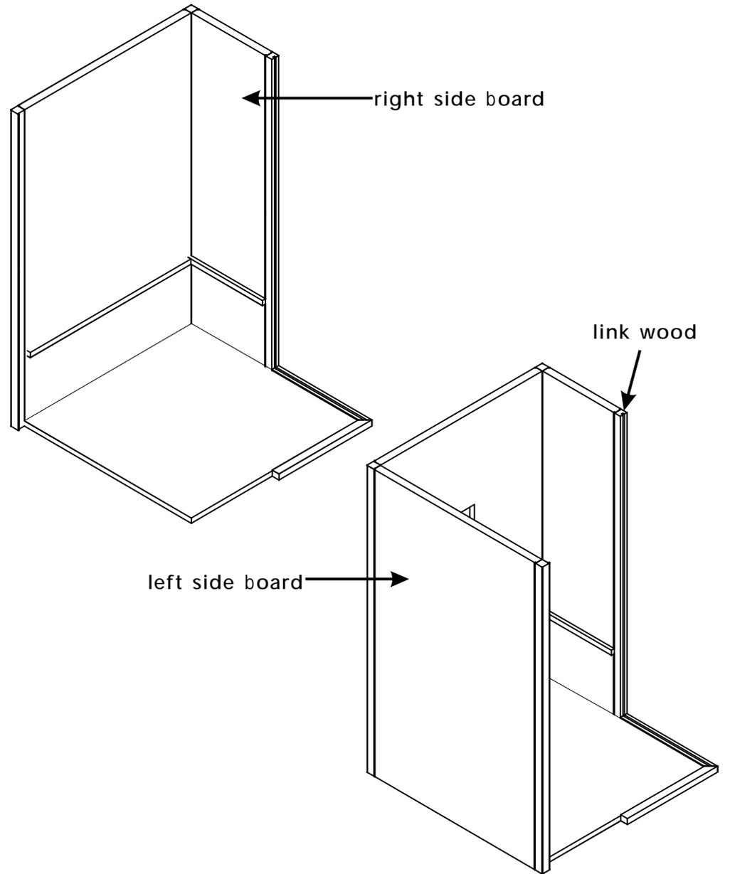
2. Same as first step, install right side board, left side board and link wood.
